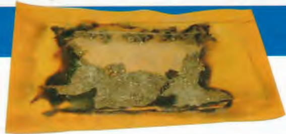
Phosphine PrePac not properly disposed of, burned.
