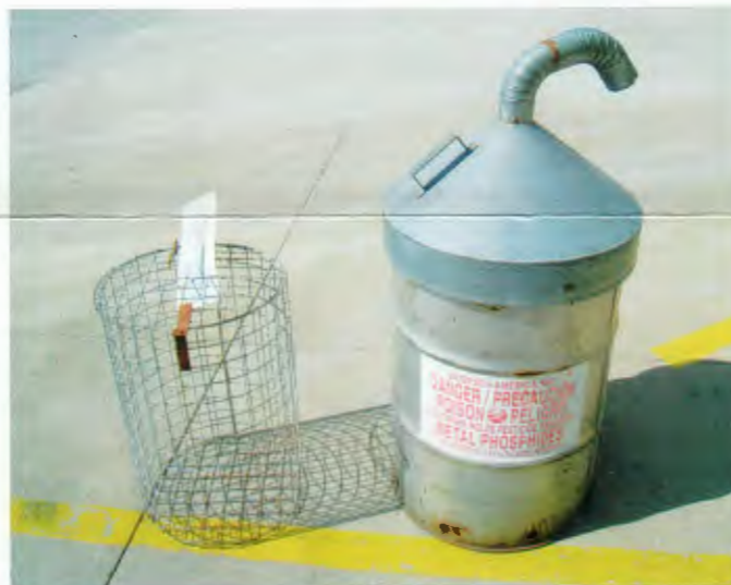
Phosphine PrePac dry de-activation system (drum) on the right and a wire disposal basket on the left.
