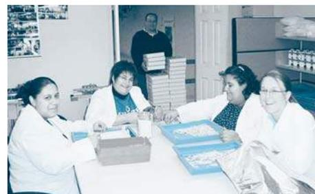
*A full time staff carefully makes each Bullet Lure to exact specification. Each Bullet Lure has seven steps to complete. Approximately one million lures were produced by Insects Limited.*
