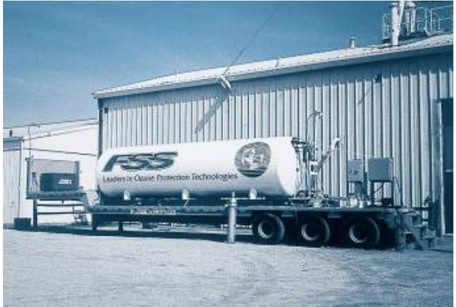
**This 24,000 lb. carbon dioxide vessel is used to fumigate structures in combination with heat and phosphine.**
