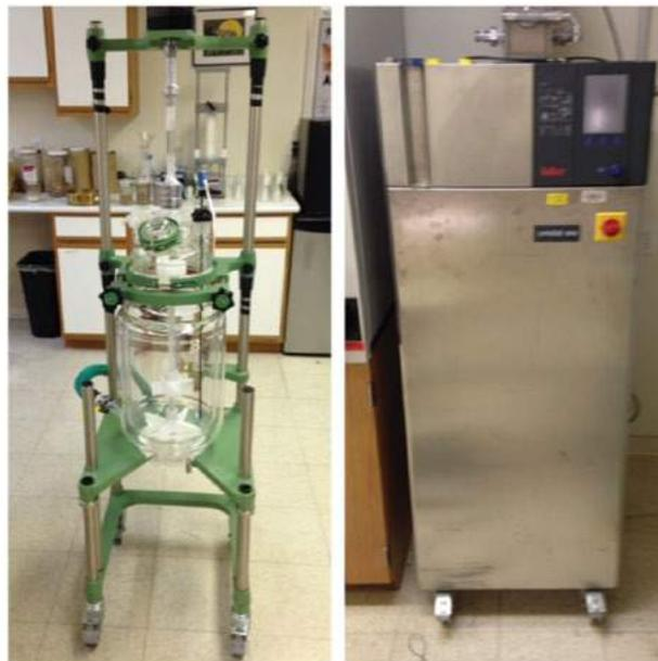
New 20 liter reactor (left) and  $-70$  degree industrial chiller (right) for pheromone production.
