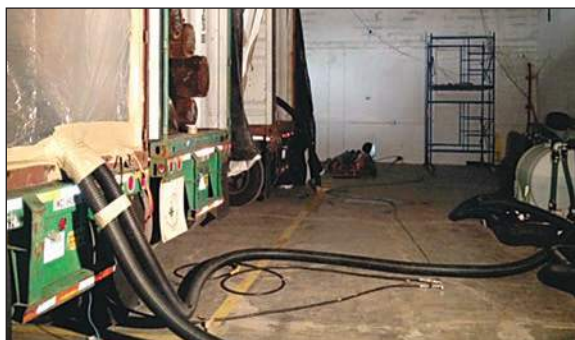
(above) Pete Swords, pheromone chemist for Insects Limited, has improved the F.A.S.T. fumigant scrubber used to destroy fumigants and improve bystander safety.
