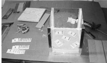
*These test boxes were placed in commercial mill fumigation using MB and SF. Gas concentrations and environmental conditions were closely observed.*
