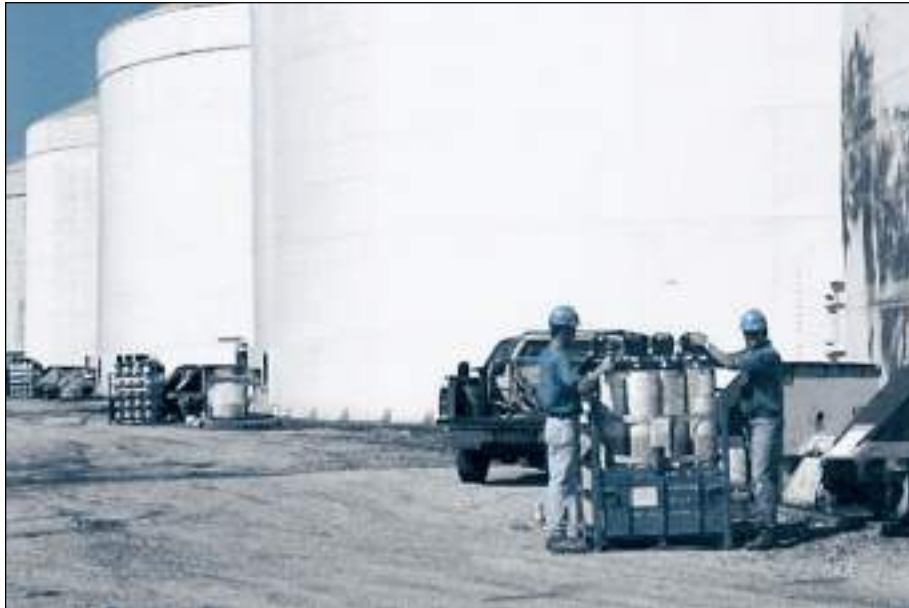
ECO 2 FUME® Phosphine fumigant being used on large grain bins in Chicago. One cylinder of ECO 2 FUME fumigant will treat 77,500 cu. ft. at 200 PPM. A pallet rack of 16 cylinders of ECO 2 FUME fumigant will treat 500,000 cu. ft. at 500 PPM. The cost is the same as magnesium phosphide and pre-packaged aluminum phosphide.
