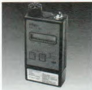
New Pac II gas monitoring device for phosphine at a range of 0 - 1.0 ppm. This device is good for personal monitoring and venting railcars. Call FSS for more information.
