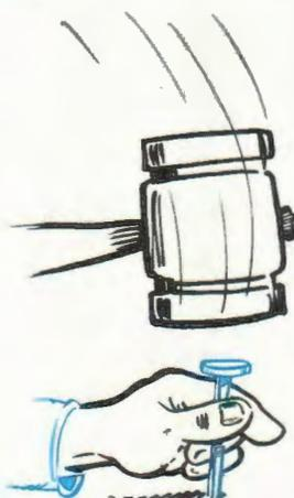
The big hammer will accomplish the job quicker but at the risk of bending the nail if the force is not directed accurately. The wall's surface could be blemished if the nail is missed or hammered too hard.
