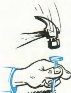
The small hammer takes more taps to sink the nail into the wall and there is less chance in bending the nail or putting a hole in the wall.
